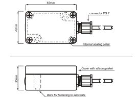
Optical sensor in convenient low dimensioned casing, to be connected by connector PG7 with round cable Ømax7 mm, (for ex. 2x0,5mm²) of length acc to necessity, Box with special sealing flange, fastened to the substrate by two screws, closed by a cover with silicon gasket and tightened by 4 screws.
